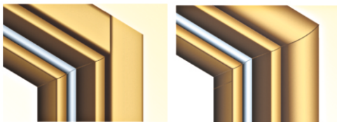
different types of joining the architraves to the door frames
